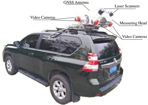
Figure 2. Acquisition system consists of two laser scanners, up to six video cameras, and a combined IMU/GNSS system.
