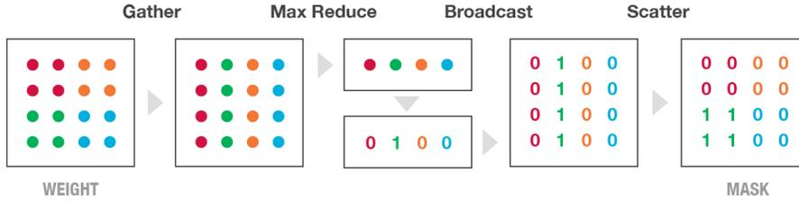
Figure 1: Generating block-sparse masks from a weight matrix
