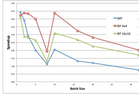
(b) Speed-up for GRU 2560 layer matrix multiply
